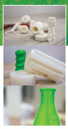
Not everything needs to be machined on an expensive CNC machine. Big savings can be gained by 3D printing components or fixtures.
